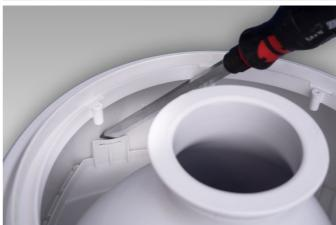
16. Loosen the bowl by carefully pushing one of the two rear fastening clips forward with a screwdriver with a long shaft. If the bowl still does not pull off well, loosen the second rear fastening clip in the same way.
