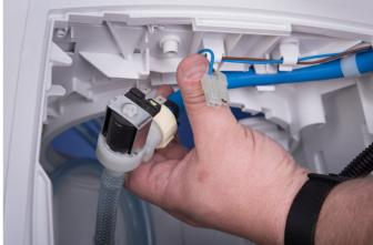
10. Disconnect the connector from the solenoid valve.
