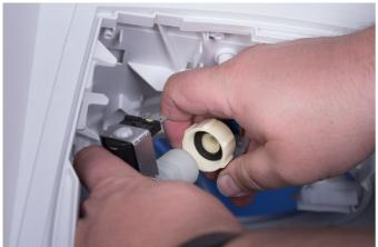
12. Disconnect the fresh water hose from the fresh water pump. Have a bucket ready to collect water standing in the hose.
