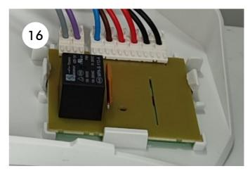
16. Remove the printed circuit board from its holder by pushing the three fastening clips outwards.
