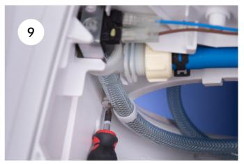
9. Unscrew the fresh water hose; it may be necessary to loosen the screws on the clamps.
