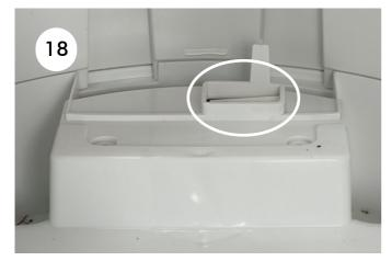
18. Put the cables with the plugs into the cable gland. You can lead the cables and plugs back at the cable harness (power supply of the toilet) and secure them there.
