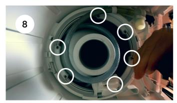
8. Through the service flap, loosen the six screws that secure the three slide bearings of the bowl of your Thetford chemical toilet to the base and remove the bearings. If necessary, turn the bowl to reach the screws.
