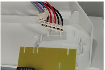
17. Remove the two connectors from the printed circuit board.
