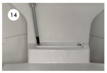
14. Loosen the two screws that secure the cover in front of the back wall of the service compartment.
