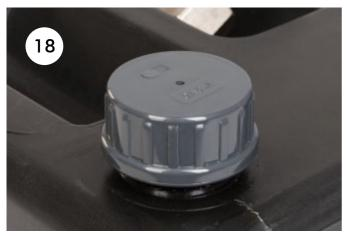
18. When transporting the liquid tank, make sure that you do not turn it upside down, as drops could then spill out of the cap of the spout. The cap is equipped with a vent to ensure pressure equalisation during use of the cassette.
