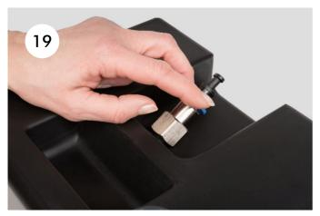
19. Before emptying, pull the plug out of the hose connection of the liquid tank again to allow for pressure equalisation.
