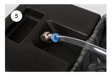
5. Push the loose end of the urine hose attached to the fluid outlet of the seat part firmly into the hose connection of the fluid tank. To make this easier, you can put the toilet in the position in which you use it. Then the hose has the maximum length and can be inserted more comfortably. Make sure that the hose is routed without kinks and with a downward slope.
